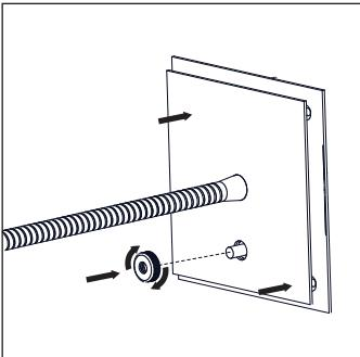
5. Carefully slide the cover plate back over the arm and into position, lining up the switch with the hole. Screw on the switch cover and tighten to secure the cover plate.
