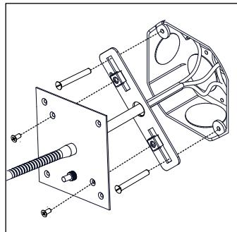
4. Adjust cable so they are inside the wall box. Attach the back plate and adapter bracket (2 gang box only) to the wall box.
