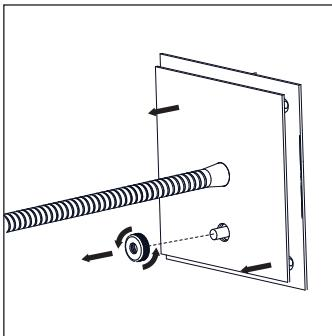
2. Unscrew the switch cover from the switch to free the cover plate. Carefully slide the cover plate over the arm to allow access to the wall plate.
