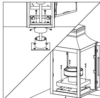
6. Place the lantern on the mounting collar, lift the wiring tray cover and tighten the security screws to the mounting plate. Tighten the 3 screws that secure the lantern to the collar of the mounting plate.
