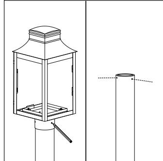
1. Open the door of the lantern and remove the glass bulb cover. Remove the screws which secure the wiring tray cover.
