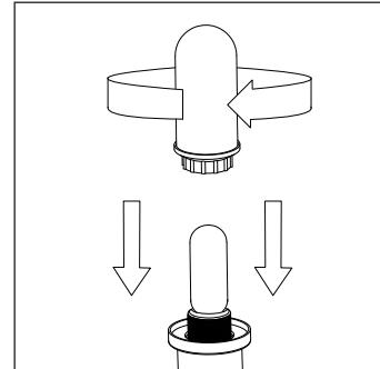
9. When the bulb has been replaced, replace the gasket and the glass cap ensuring the cap is secured tightly.
