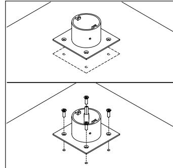
3. Mark and drill the locations of the mounting holes. Ensure that the supply cable is in place and then secure the mounting plate to the surface using suitable fixings. Caulk (Silicone Caulking Compound, not supplied) completely around the contact section of the mount to prevent water ingress.
