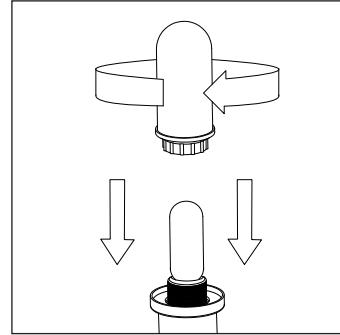
9. When the bulb has been replaced, replace the gasket and the glass cap ensuring the cap is secured tightly.
