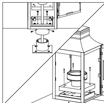
4. Replace the wiring tray cover removed earlier. Ensure the supply wires are protruding from the wiring hole in the base of the lantern. Ensure that the rubber seal is in place around the top of the wiring tray.
