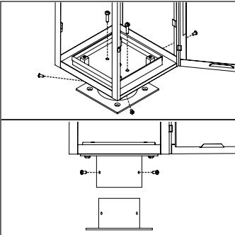
2. Remove the security screws that hold the lantern onto the base. Remove the screws on the mounting collar and lift the lantern off from the mounting collar base.
