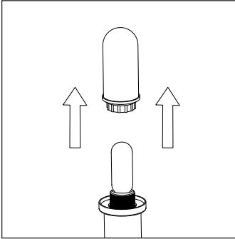
8. To replace the bulb, unscrew the glass cap on the lamp holder and remove the bulb.
