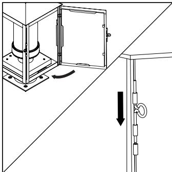
10. After accessing the bulb, gently close the door. Close the latch and ensure it is secure.
