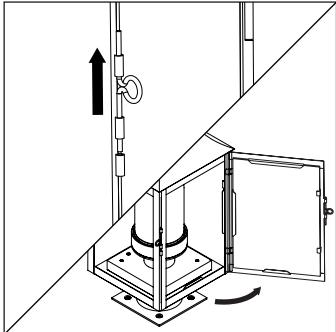
7. To access the bulb, pull the latch to release the door.
