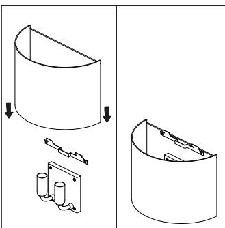
5. Place the lampshade above the lampshade bracket and carefully mount into place.
