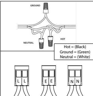
5. Having identified the household wiring, connect the building supply and the product cables together in the wire connectors as shown above.
