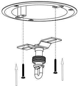
1. Attach the bracket to the Ceiling Box ensuring it is secured tightly.
