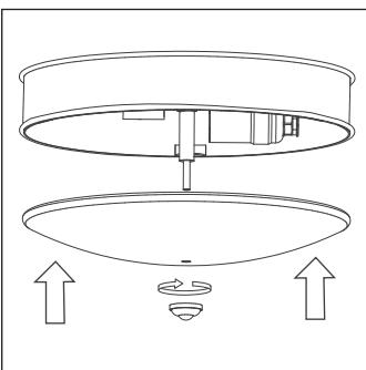
5. Carefully replace the glass and screw the finial back on to complete installation.
