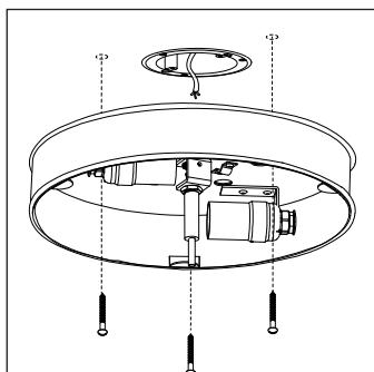
4. Using Suitable fixings, secure the light to the ceiling using the mount holes.
