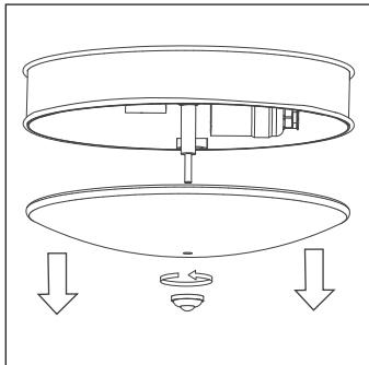
1. Unscrew the finial and carefully remove the glass.
