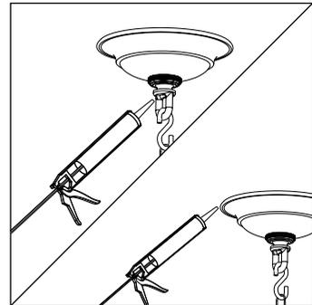
6. Apply a 3mm bead of silicone around the perimeter of the ceiling rose & cable exit hole. Ensure there is a complete seal between all surfaces.
